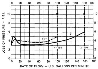
NOTE: • Maximum allowable pressure loss allowed by USC at indicated flow.
