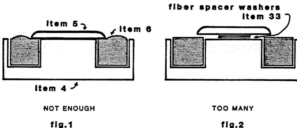
In Fig 1 above, ADD fiber spacer washers (item 33) between the disc guide (item 5) and disc retainer (item 4), until bulge disappears, but disc cannot be rotated.
