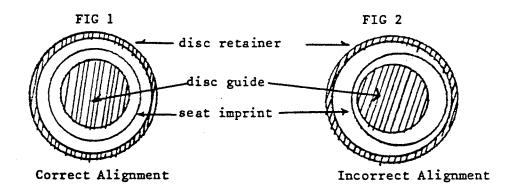
In the event the seat imprint resembles FIG. 2, adjust hinge pin bushing OUT, on side corresponding to least distance between seat imprint and disc guide. In FIG 2 above, adjust hinge pin bushing on your RIGHT out. (For proper perspective, assume that you are looking into the inlet check valve).
